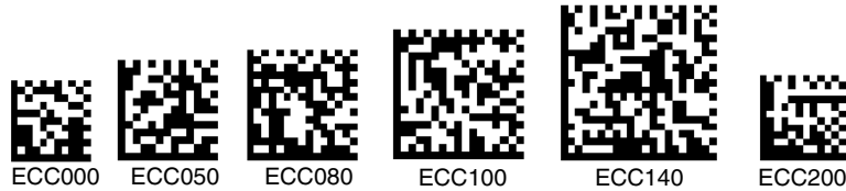
FIGURE D-5. Data Matrix Examples with Different ECC Levels
